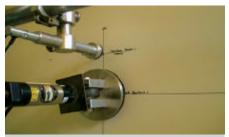
500N static horizontal point load at 1500mm height. (500N = 50Kg = 2 bags plaster
