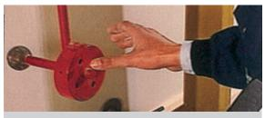
**Surface Damage /Perforation** - A 3Kg impactor, with its head being a 50mm diameter steel sphere, is swung 10 times against the face of the partition.
