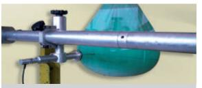
**Damage** - Partition is subjected to two impacts from 400mm diameter canvas bag filled with glass beads of 50Kg, swung against the face of the partition. **Structural** Damage - Partition is subjected to three impacts of greater energy on the stud and between the studs.
