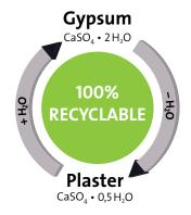
Gypsum is an inherently sustainable material as it can be completely recycled an infinite number of times. Removing water from gypsum rocks through dehydration produces a plaster powder scientifically known as calcium sulphate. This process is totally reversible: adding water reproduces gypsum.
