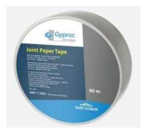
**Characteristics:** Gyproc® joint paper tape has center crease, chamfered edges and spark perforation, for easy use in all joints. It is manufactured from cross fibered paper which provides excellent crack-resistance.
