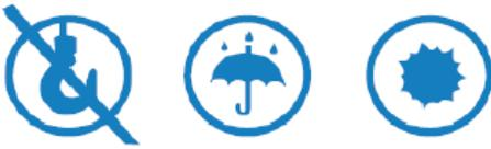
Gyproc Supreme-80 is supplied in 25Kg bags. The dimensions of the bag ensure that a well-filled appearance is presented when filled and the bags can be stacked on a pallet in a stable and well-stacked array. Bags should be stored dry, as absorption of water shortens the setting time, causes set lumps to form in the bags and may reduce the strength of the set plasterwork. No hooks or any sharp tools should be used to carry bags from one location to another.
